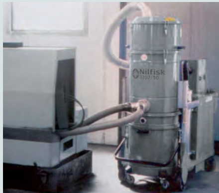
Fixed application for recovery of graphite
