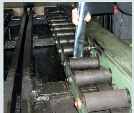
Vacuuming grinding sludge
