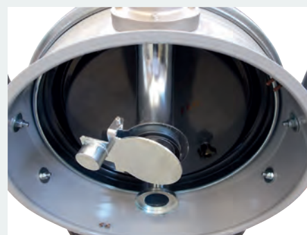
Deflector with metal flap for closing the suction during the discharge phase
